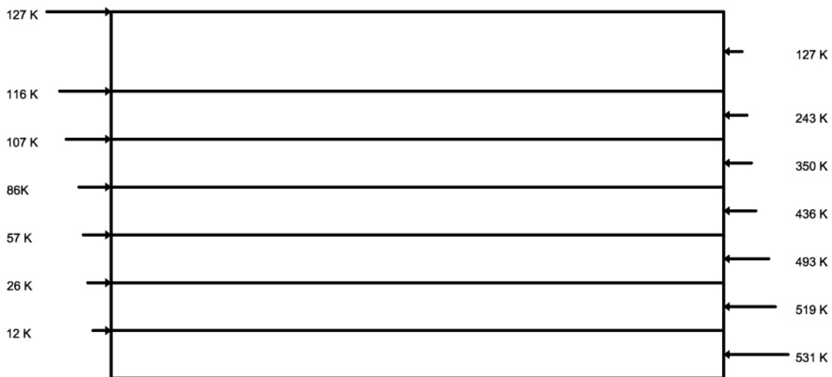
Figure 7. North Building Seismic Force Diagram
